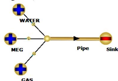
Figure 4. Maximus model for the calculation of hydrate dissociation curves
