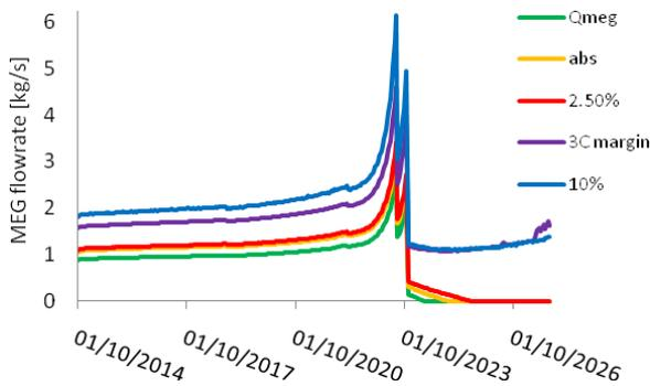
Figure 13. Comparison between MEG flowrates with different errors for the Raven trunkline
