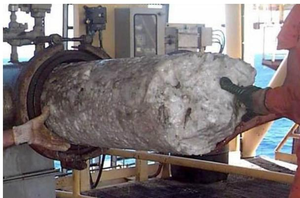
Figure 2. A large gas hydrate plug formed in a subsea hydrocarbon pipeline [Photo courtesy of Petrobras]
