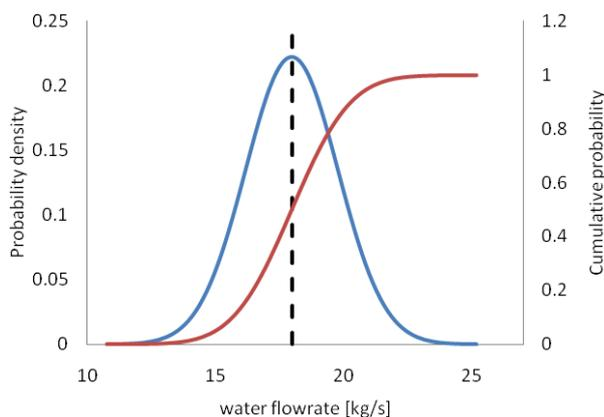
Figure 10. Uncertainty on water flow rate measurement
