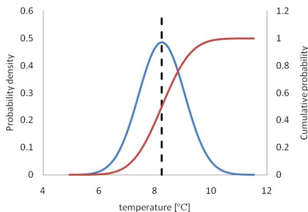
Figure 12. Uncertainty on temperature measurement
