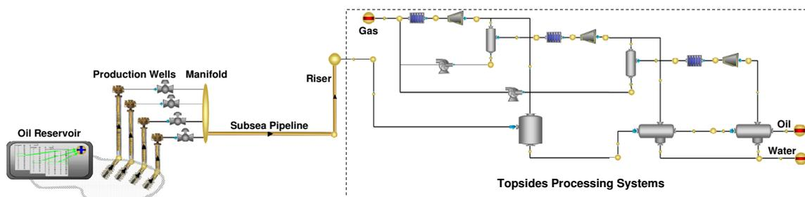
Fig. 1: Subsea Production System with Processing Facilities
