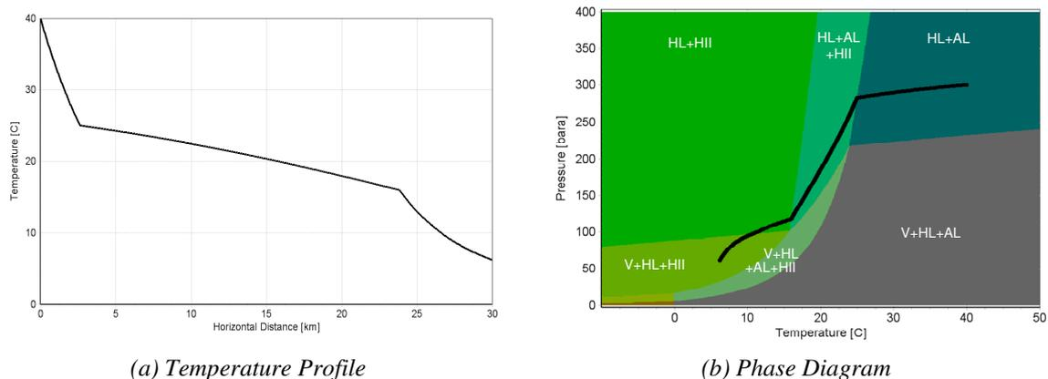
Fig. 3: Flow in Uninsulated Subsea Pipeline
