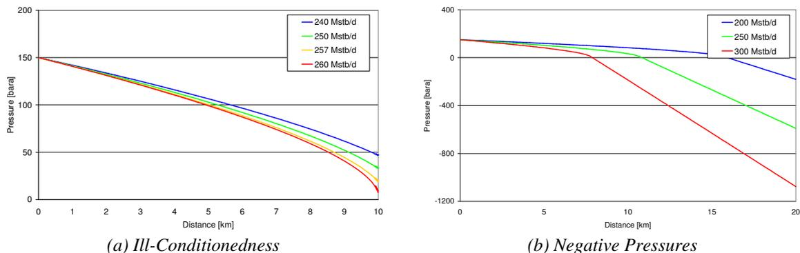
Fig. 4: Pipeline Pressure Profile Results
